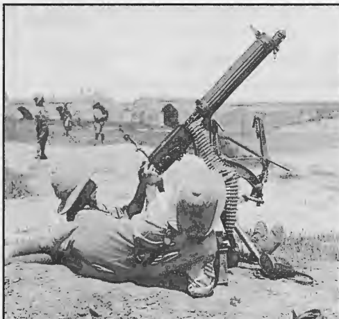
Machine gunners firing at a Turkish airplane at Hari Kupri during World War II. The tripod is fitted with the infrequently seen "overbank" cradle. Reversing the gun on the tripod was the most common form of AA mounting. Photo: Imperial War Museum
